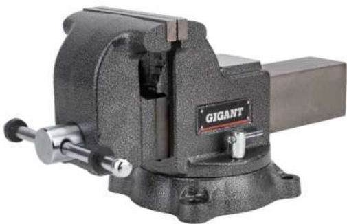
PROFESSIONAL SWIVEL MACHINIST'S VISE Professional Swivel machinist's vise 150 mm GP-BV-150
